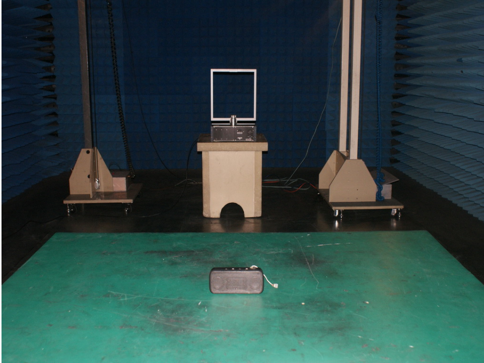
Photograph 2: Set-up for Spurious Emissions (30MHz-1GHz)
