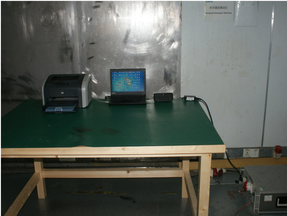
Photograph 6: Set-up for Radiated Emissions, below 1GHz
