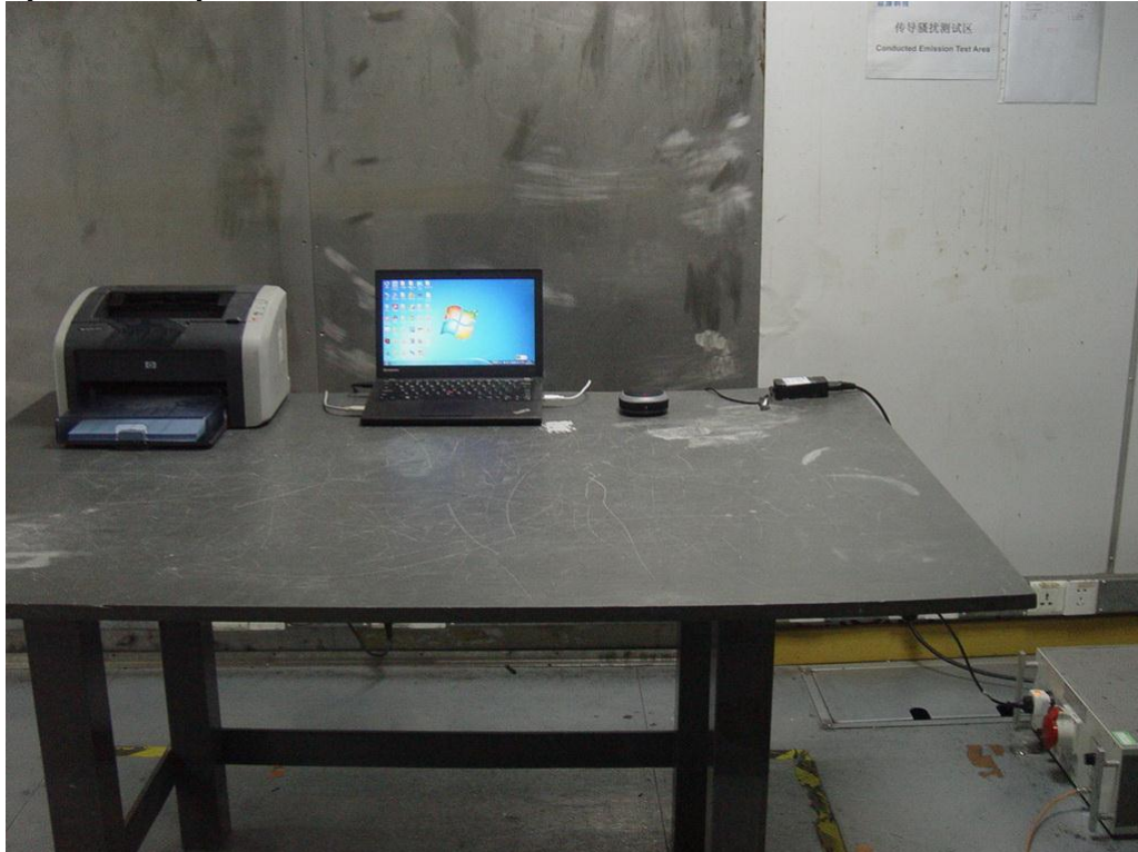
Photograph 2: Set-up for Radiated Emission of below 1GHz
