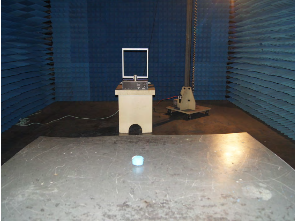
Photograph 2: Set-up for Spurious Emissions (30MHz-1GHz)
