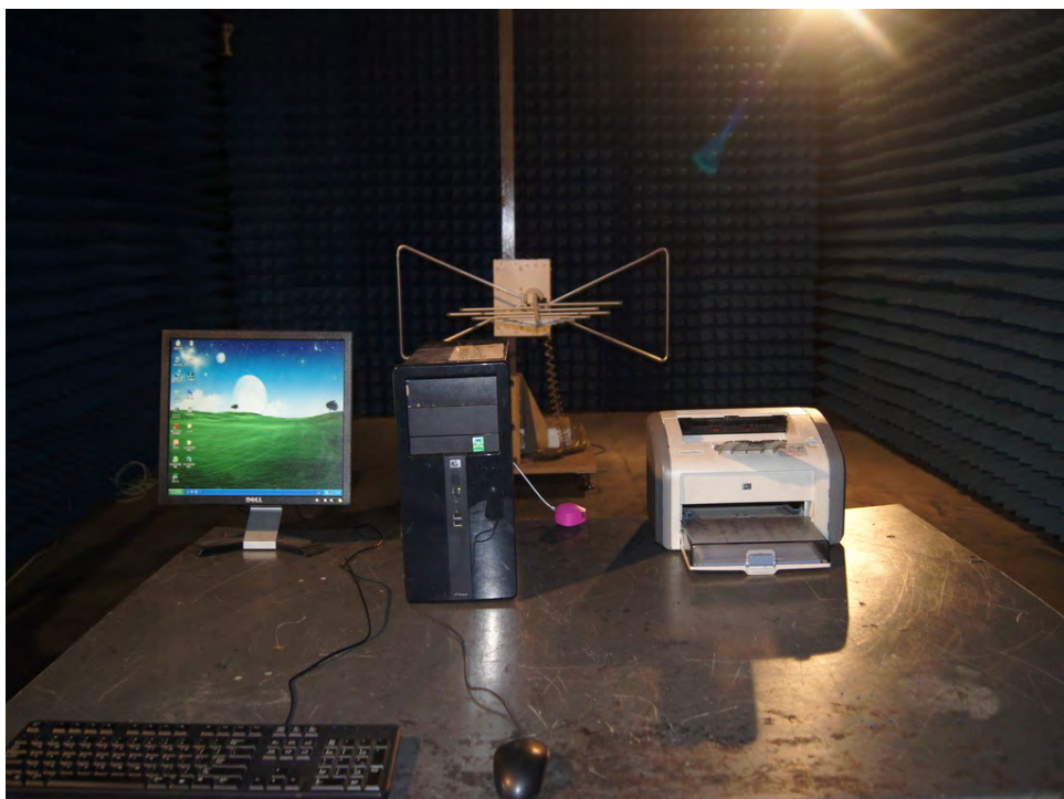
Photograph 6: Set-up for Radiated Emissions, below 1GHz
