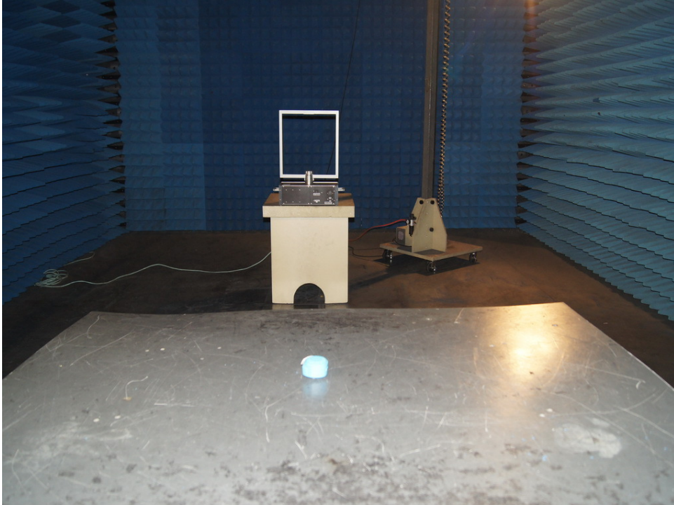
Photograph 2: Set-up for Spurious Emissions (30MHz-1GHz)
