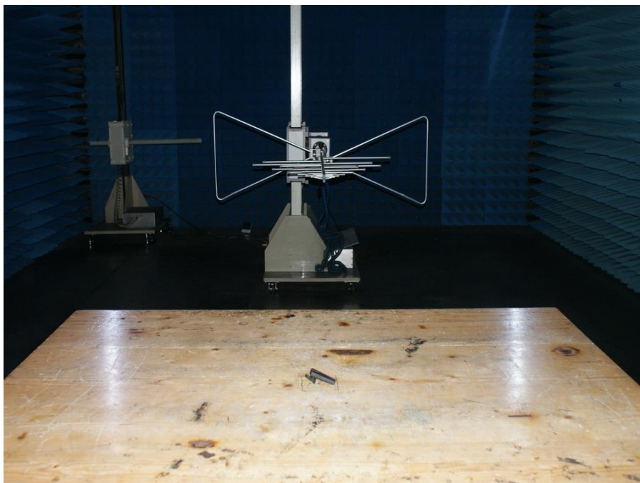
Photograph 3: Set-up for Radiated Spurious Emission, 30MHz - 1GHz
