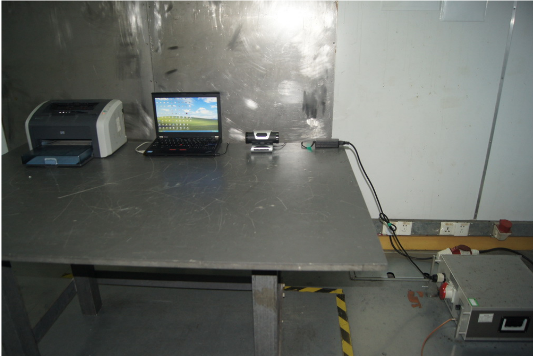
Photograph 6: Set-up for Radiated Emissions, below 1GHz
