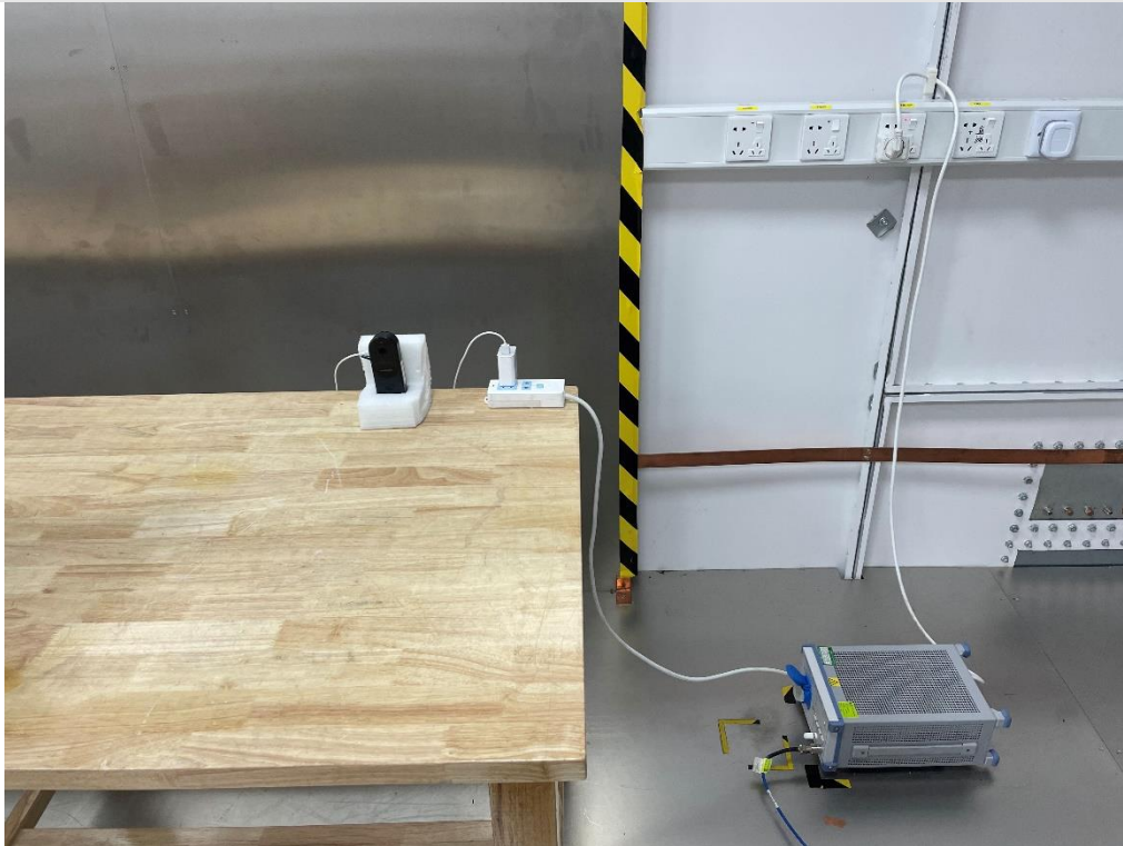
AC Power Line Conducted Emission
