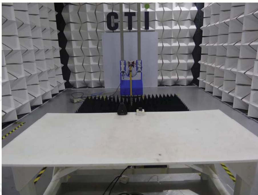
TEST SETUP OF RADIATED EMISSION (above 1GHz)
