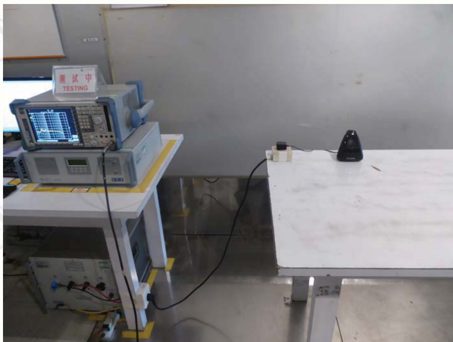
TEST SETUP OF CONDUCTED EMISSION
