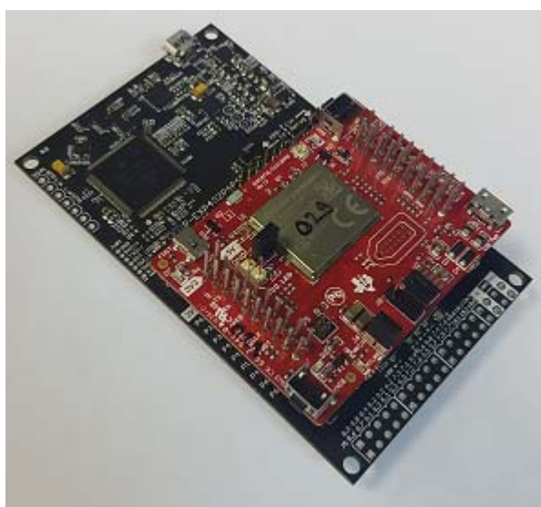
Figure 7-9: BOOSTXL-CC3120MOD Connected to MSP432 LaunchPad
