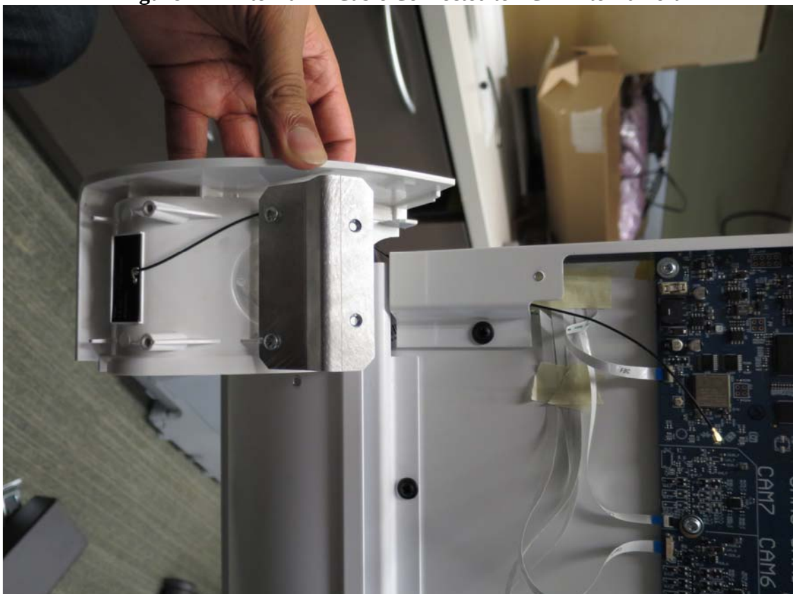
Figure F -Antenna Mounted on Front Right Bottom Corner Plastic Cover
