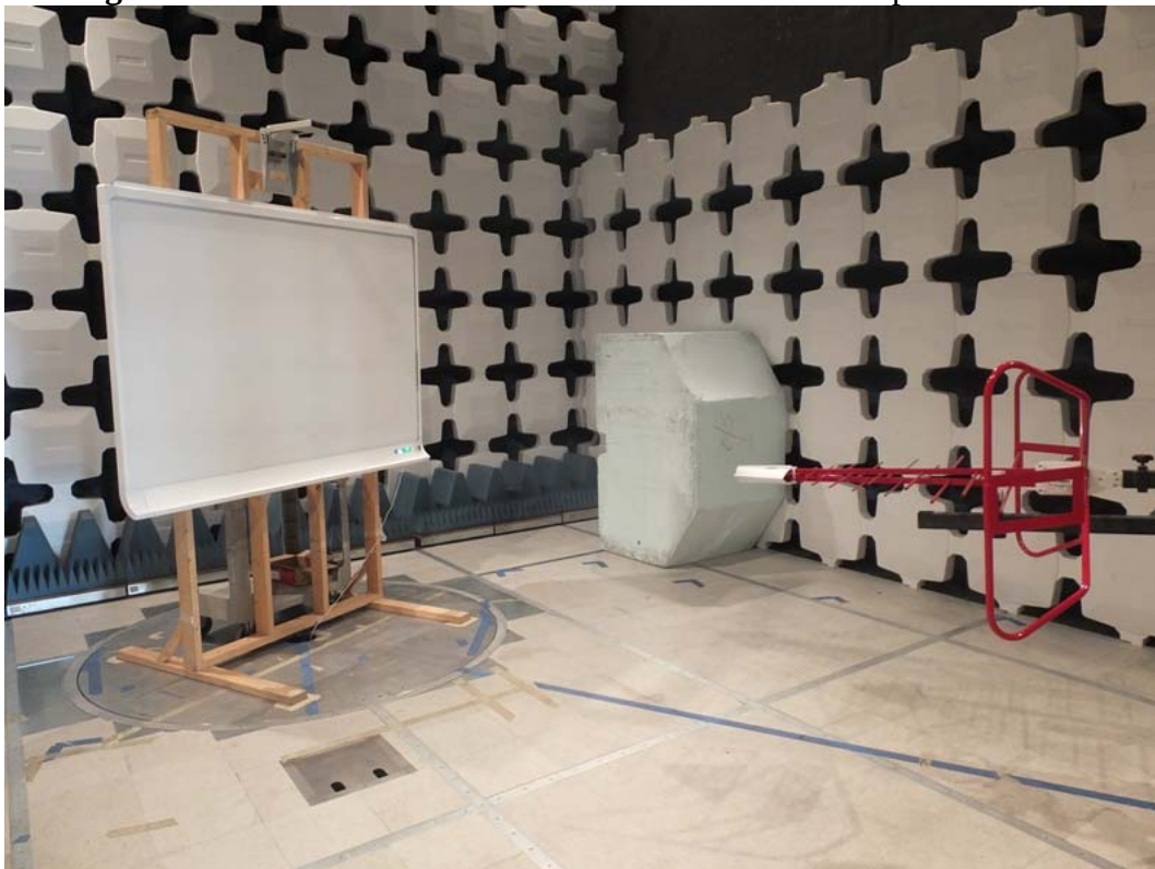
Figure 4.4B – Radiated Emissions 30M-1000M Test Setup - Side View
