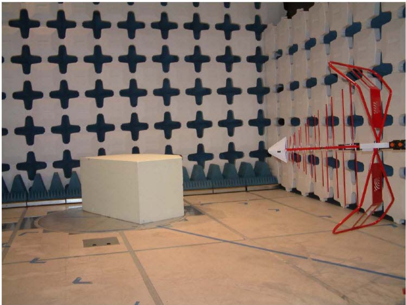
Figure 3.1 – Test Facility (setup for 30 MHz – 1GHz)
