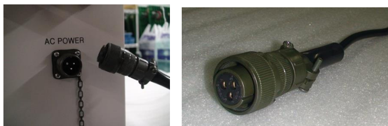
Figure 3-7 Power cable connection (AC type)
