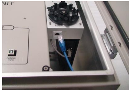
Figure 3-6 Power cable connection (PoE type)
