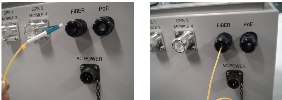
Figure 3-8 LC/UPC fiber connector connection
