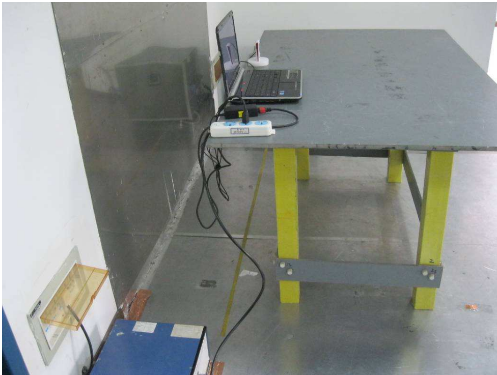
Conducted Emissions - Side View (Charging & Downloading)
