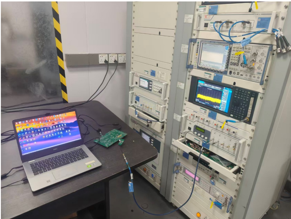
RF connect EUT antenna terminal test
