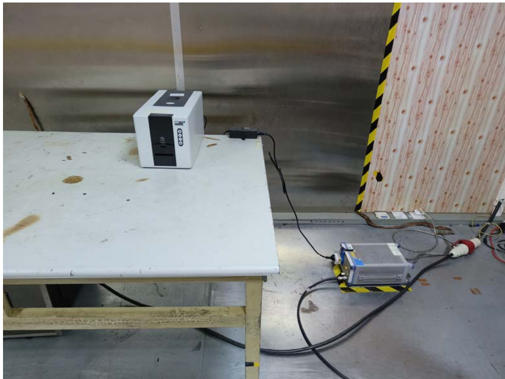
M/N: DC-2300 Conducted Emissions Test
