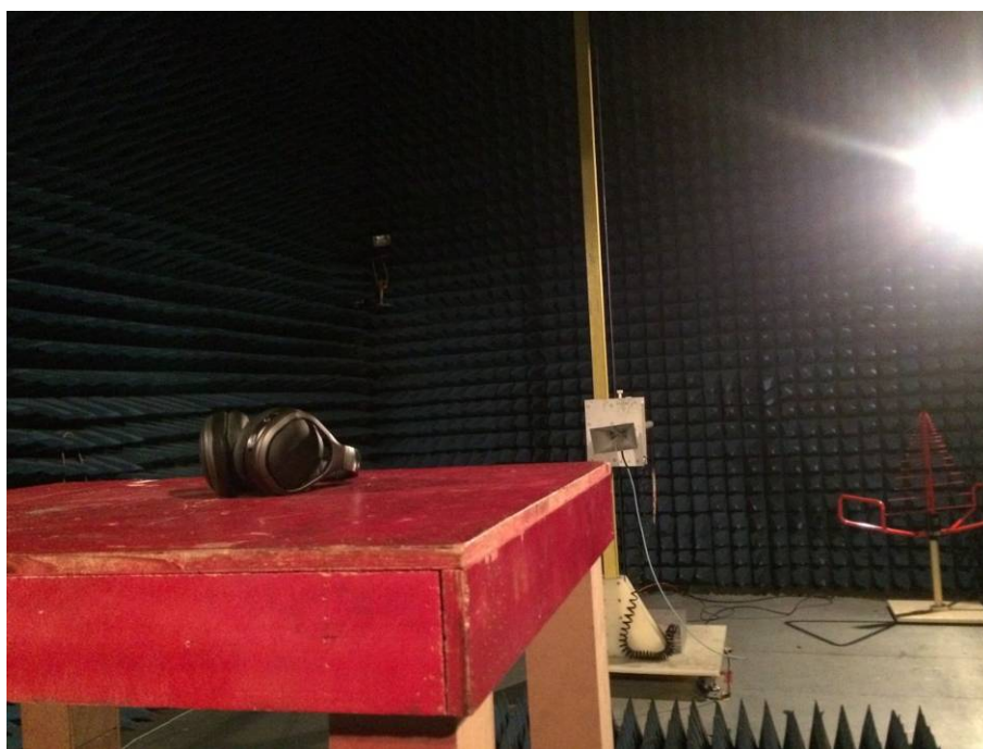
RADIATED EMISSION TEST SETUP (ABOVE 1 GHz) FROM 1.5M-HEIGHT TEST TABLE
