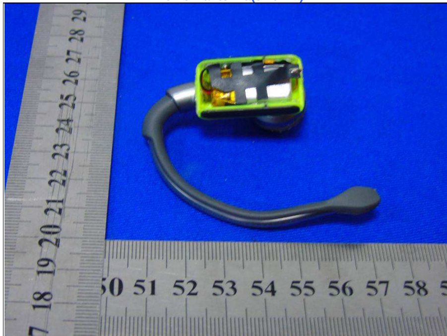
The new antenna(3M9471)
