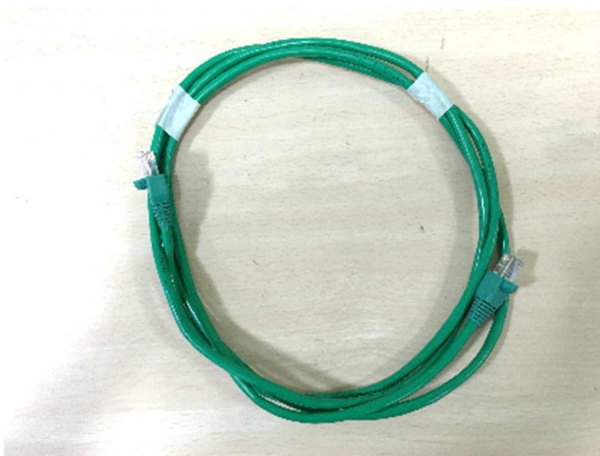
Figure 10 Photograph of RJ45 POE cable
