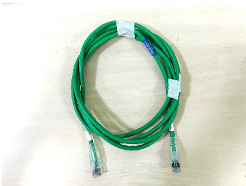
Figure 11 Photograph of RJ45 Data cable
