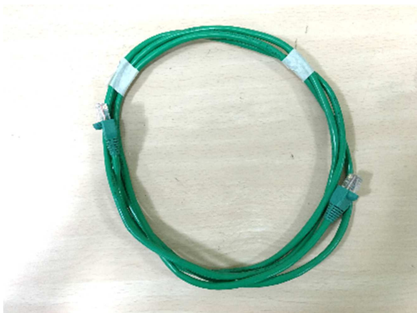
Figure 9: Photograph of RJ45 POE cable
