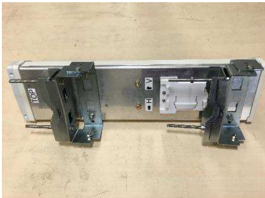
Figure 4: Photograph of 17 dBi Transmitter Antenna-Back view
