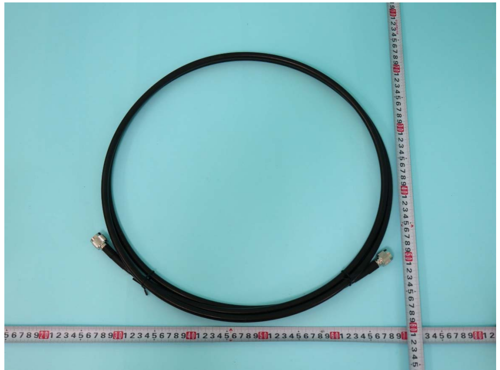
Antenna cable 1 (For Antenna Set 3~5 use)
