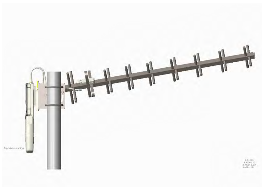
Figure 152: Yagi antenna alignment - upward tilt
