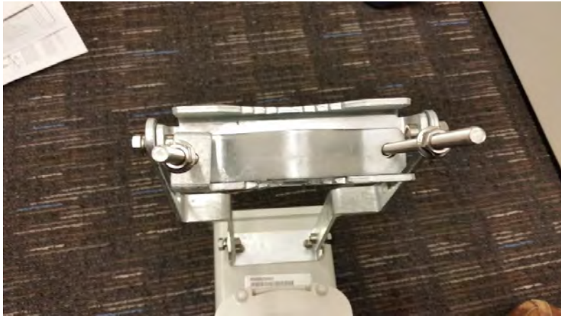
Figure 125: Assembled upper bracket connected to AP antenna
