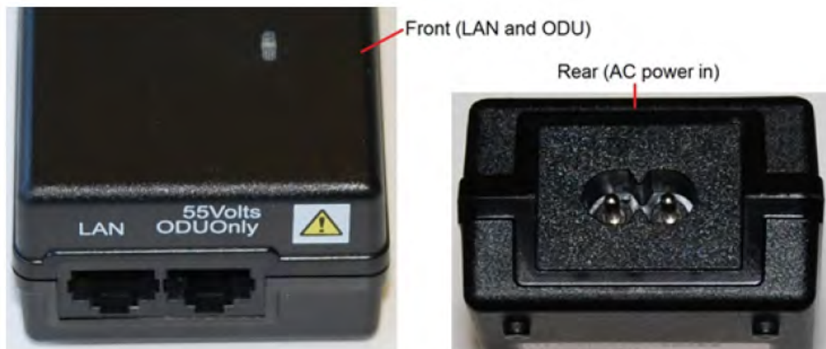
Figure 37 : AC power injector interfaces
