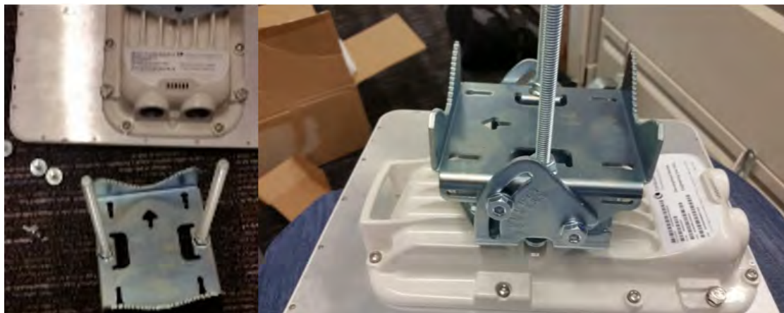
Figure 155: Attaching the bracket body
