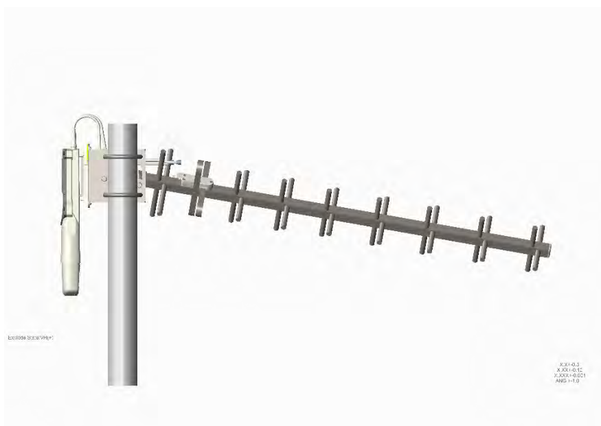
Figure 153: Yagi antenna alignment - downward tilt
