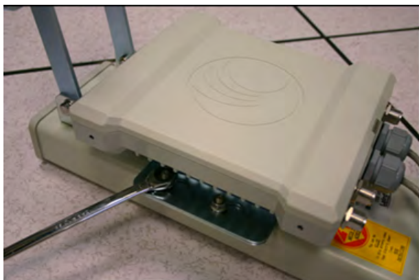
Figure 137: Lower bracket attached to AP antenna
