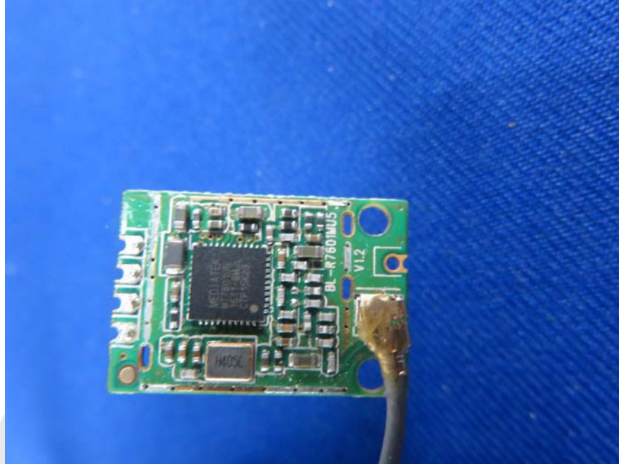
8. Figure PCB of the RF board-Back View
