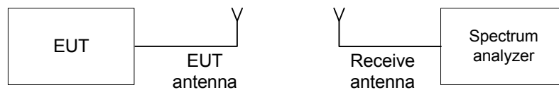
Figure 7.2.1 Occupied bandwidth test setup
