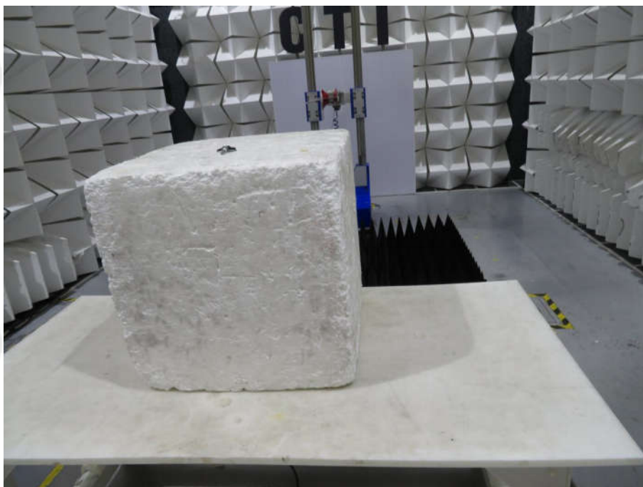
Radiated spurious emission Test Setup-3(Above 1GHz)
