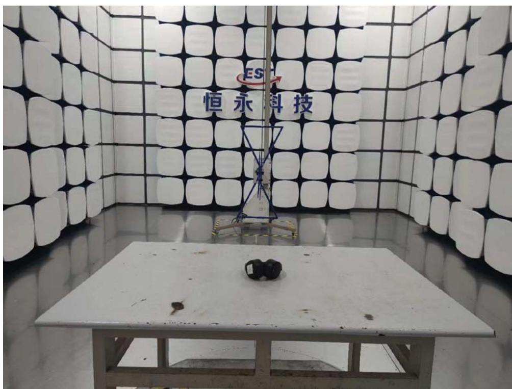
Radiated emission test: Below 1GHz
