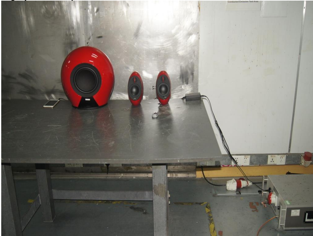
Photograph 2: Set-up for Spurious Emissions for below 30MHz
