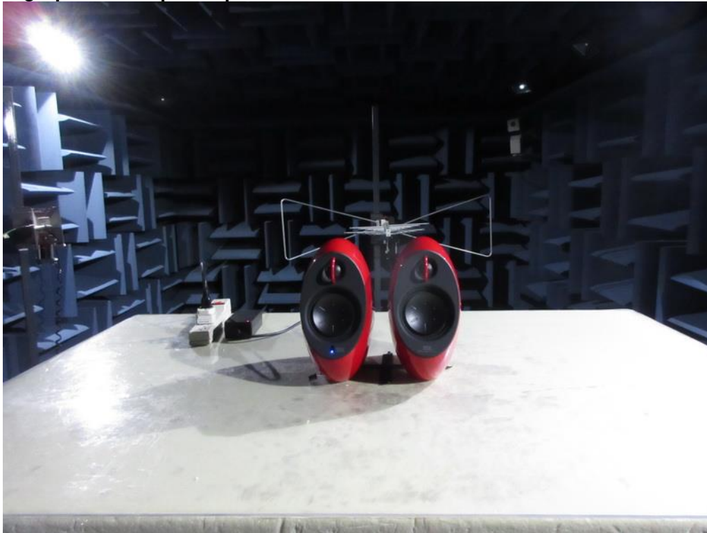
Photograph 4: Set-up for Spurious Emissions for 1 - 18GHz
