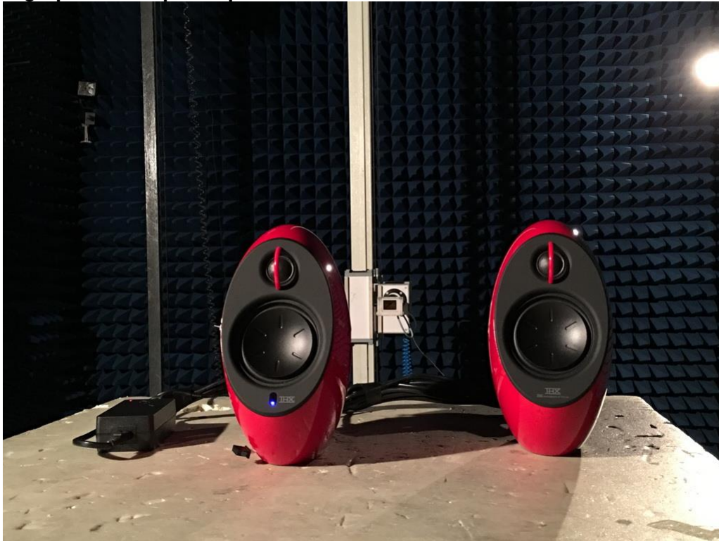
Photograph 6: Set-up for Spurious Emissions for 26.5 - 40GHz
