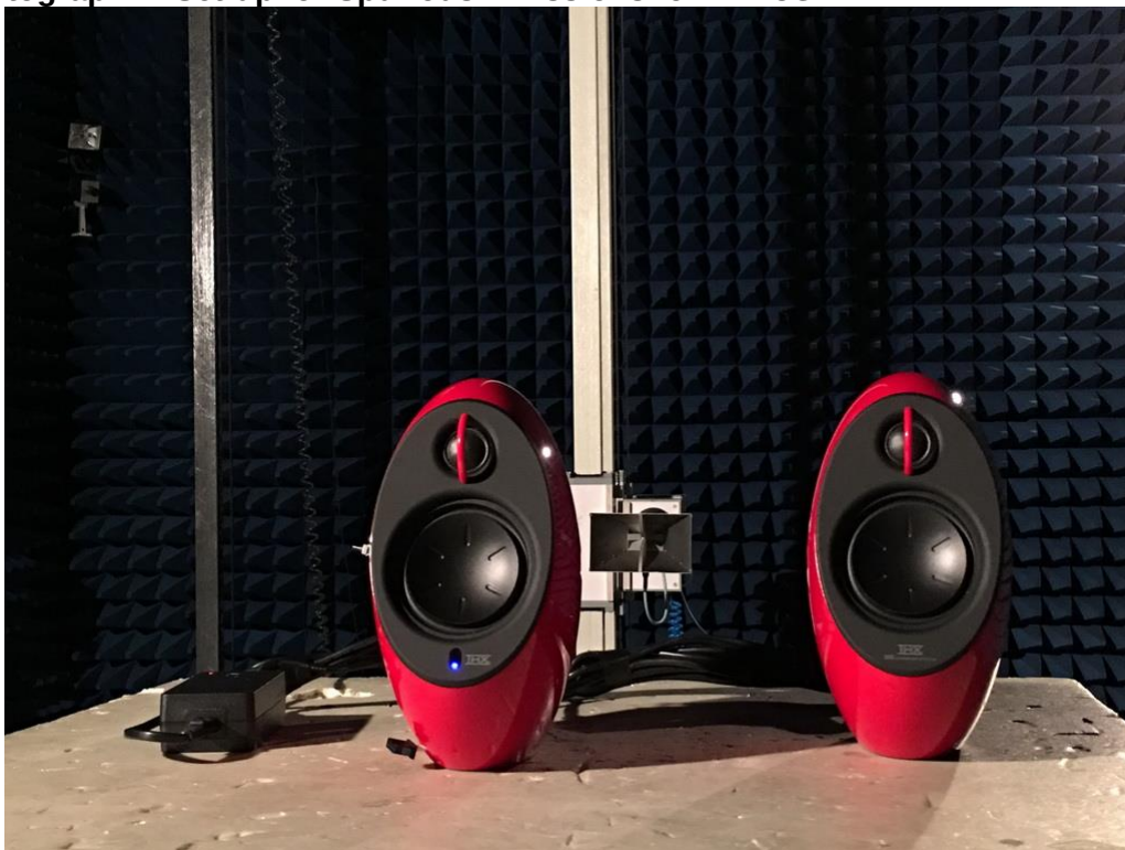
Photograph 4: Set-up for Spurious Emissions for 1 - 18GHz
