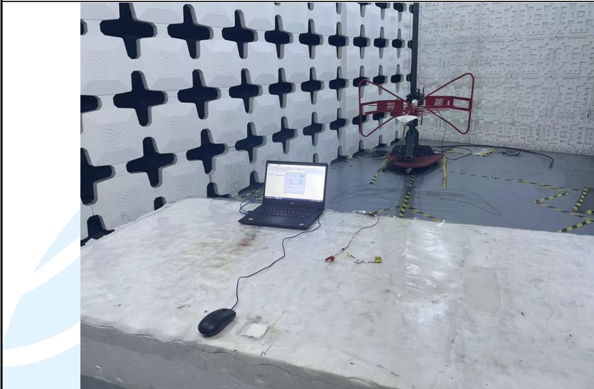
Radiated emission Test Setup (30 MHz~1 GHz)_ Left Ear
