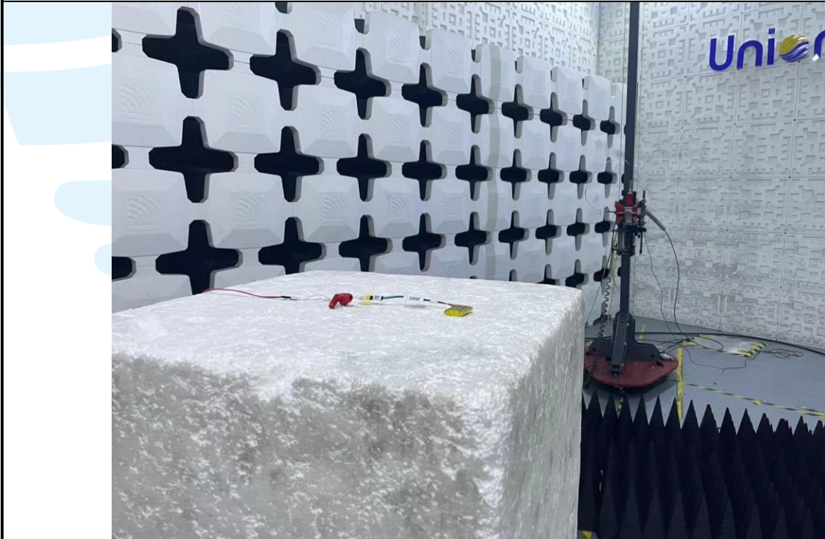
Radiated emission Test Setup (Above 1 GHz) _ Right Ear
