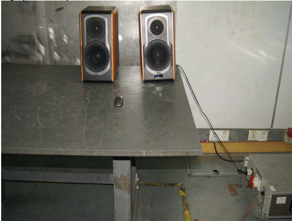
Photograph 2: Set-up for Spurious Emissions for below 30MHz
