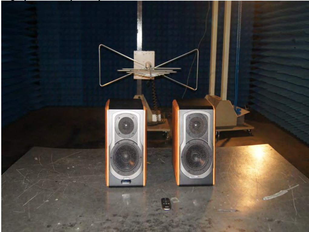
Photograph 4: Set-up for Spurious Emissions for 1 - 18GHz
