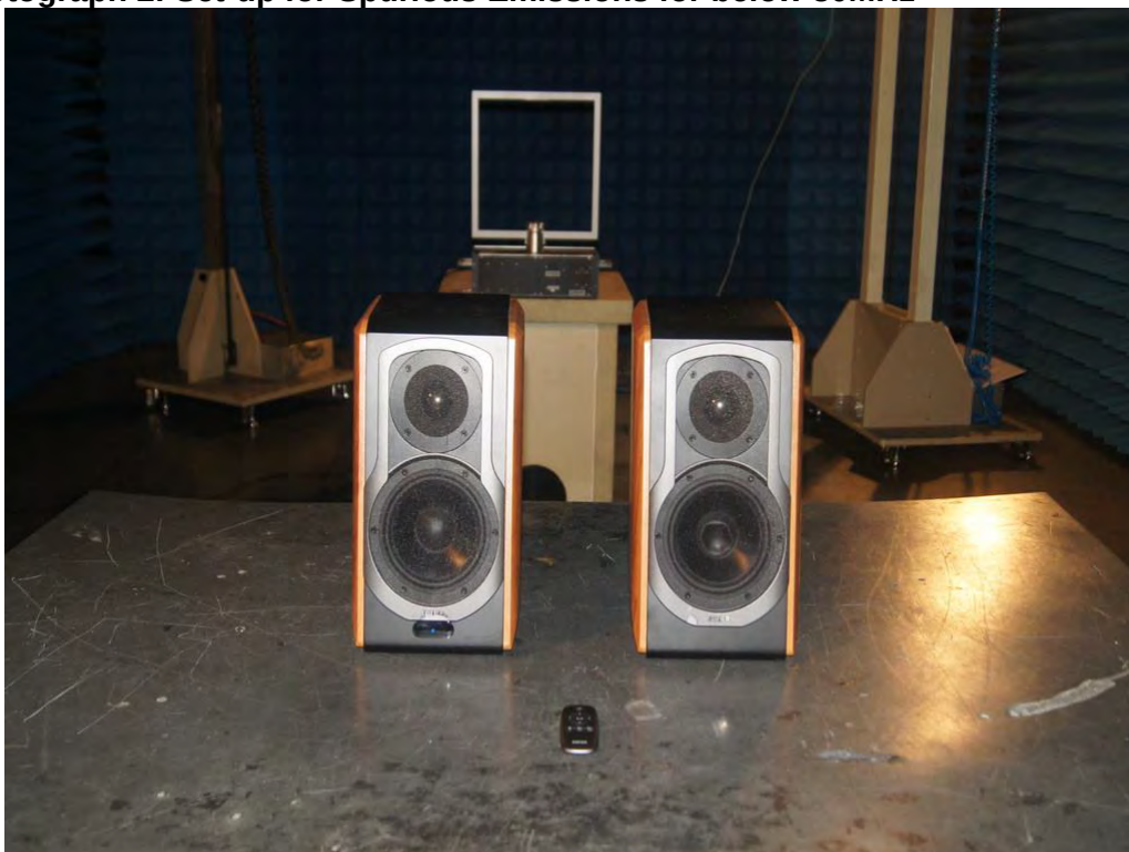
Photograph 2: Set-up for Spurious Emissions for below 30MHz
