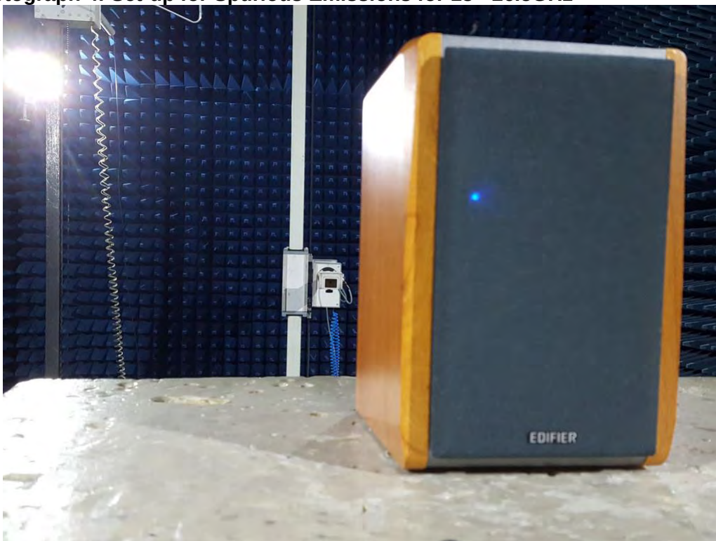
Photograph 4: Set-up for Spurious Emissions for 18 - 26.5GHz
