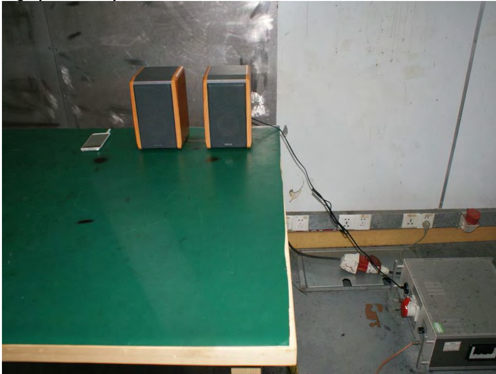
Photograph 6: Set-up for Radiated Emissions
