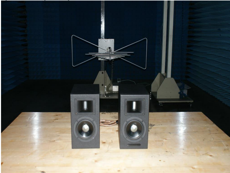
Photograph 2: Set-up for Spurious Emissions for 30 - 1000MHz
