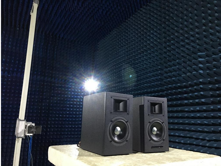
Photograph 4: Set-up for Spurious Emissions for 18 - 26.5GHz
