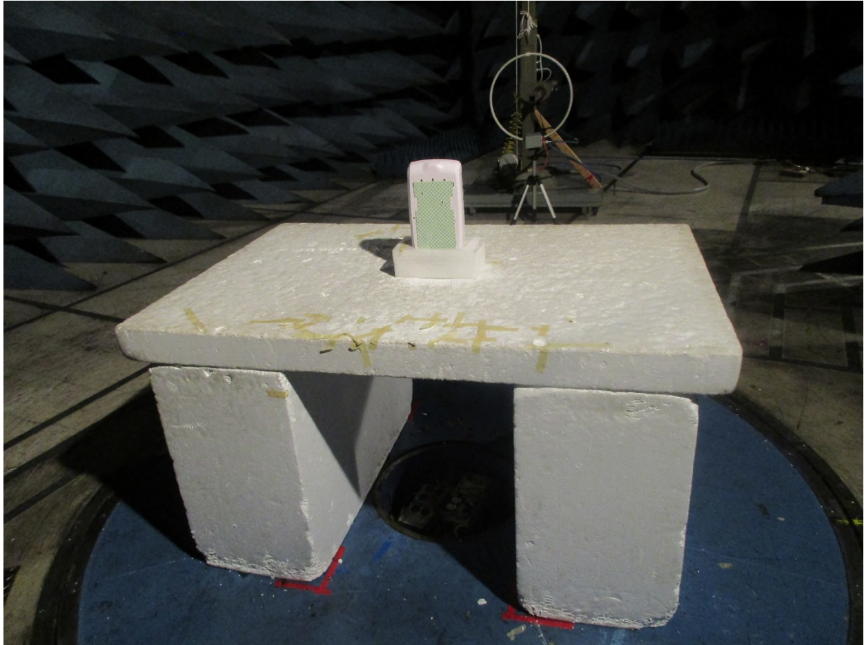
Figure 2: Radiated Emissions – Back View – 9 kHz – 30 MHz
