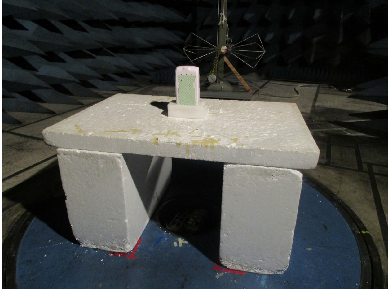
Figure 3: Radiated Emissions – Back View – 30 MHz – 200 MHz
