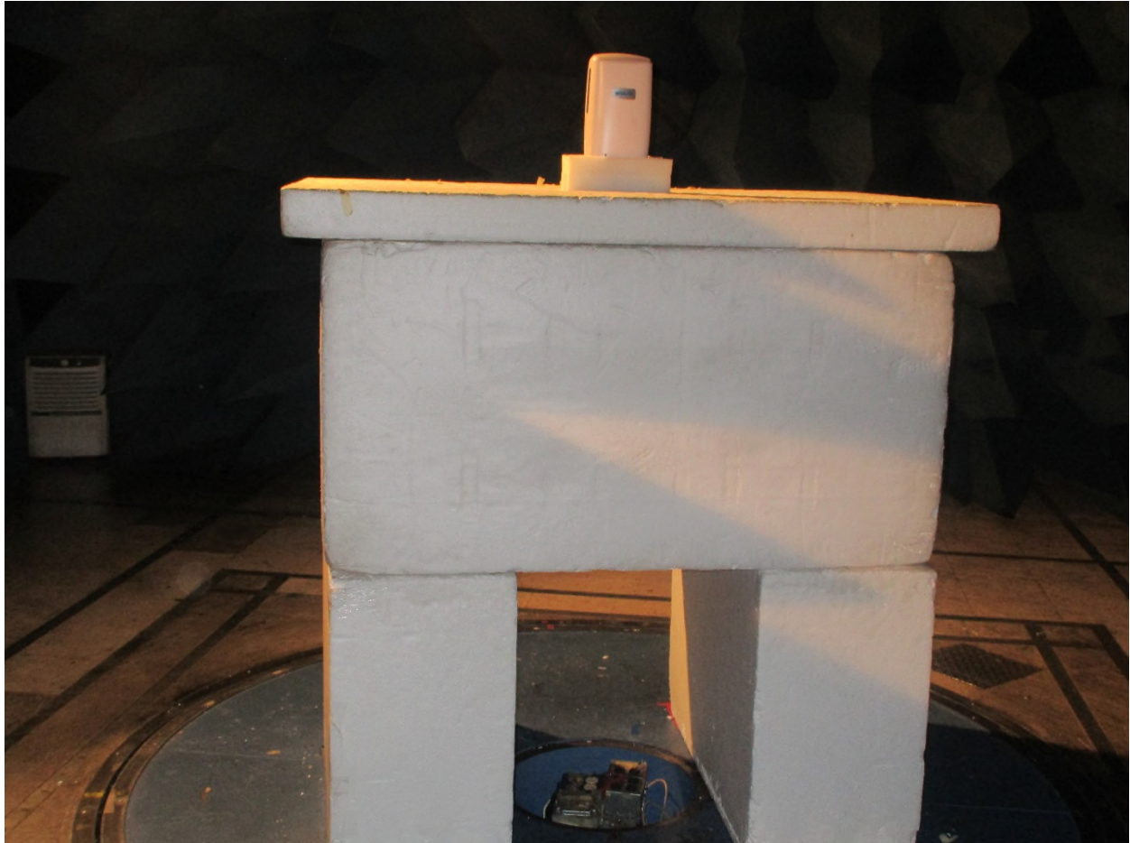
Figure 5: Radiated Emissions – Front View – Above 1 GHz
