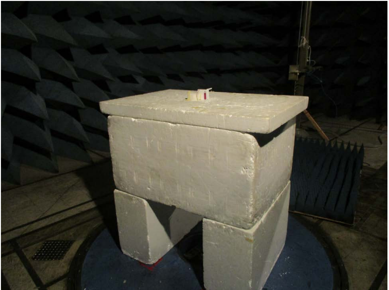
Figure 6: Radiated Emissions – Back View – Above 1 GHz
