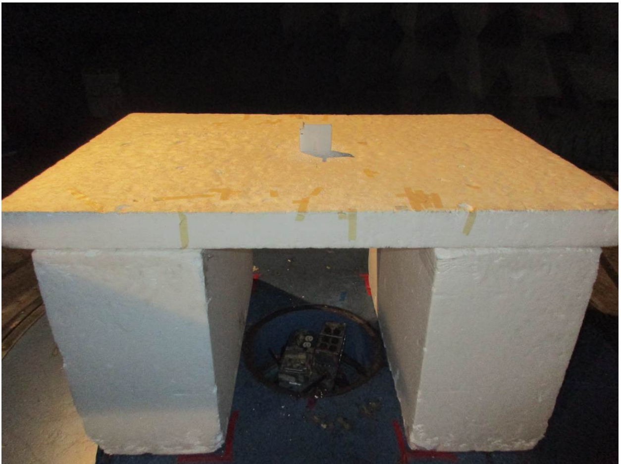
Figure 1: Radiated Emissions – Front View – Below 1 GHz
