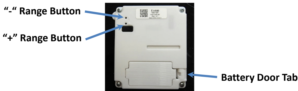
Figure 2. Back view, showing, battery door tab, and range button locations
