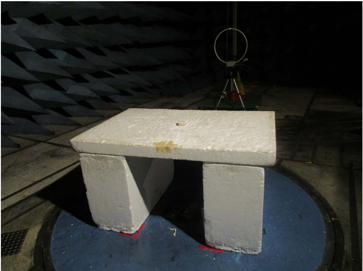
Figure 1: Radiated Emissions – EUT Standing – below 30 MHz
