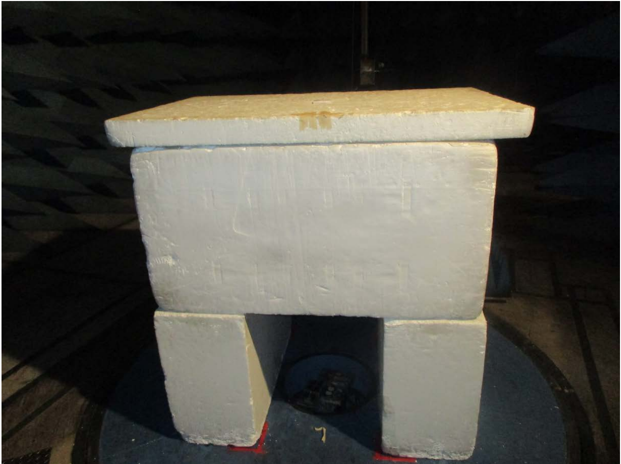
Figure 5: Radiated Emissions – EUT Flat – above 1 GHz
