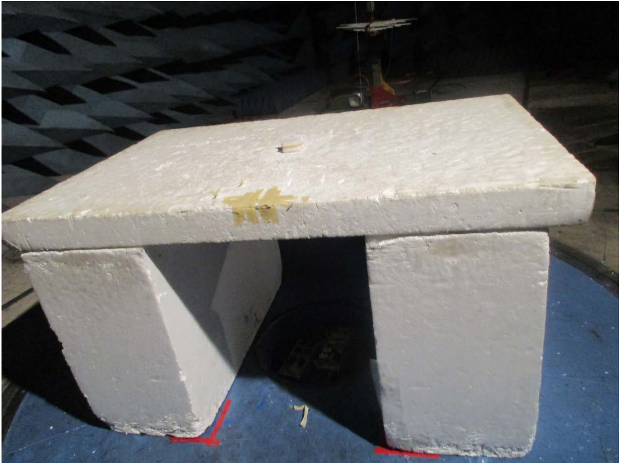
Figure 3: Radiated Emissions – EUT Standing – 200 MHz – 1 GHz
