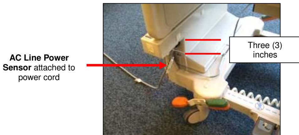
Figure 7. AC Line Power Sensor Attached to Power Cord
