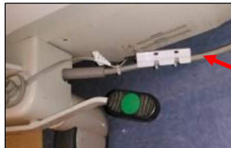
Figure 3. The AC Line Power Sensor Installation Location on the Bed
