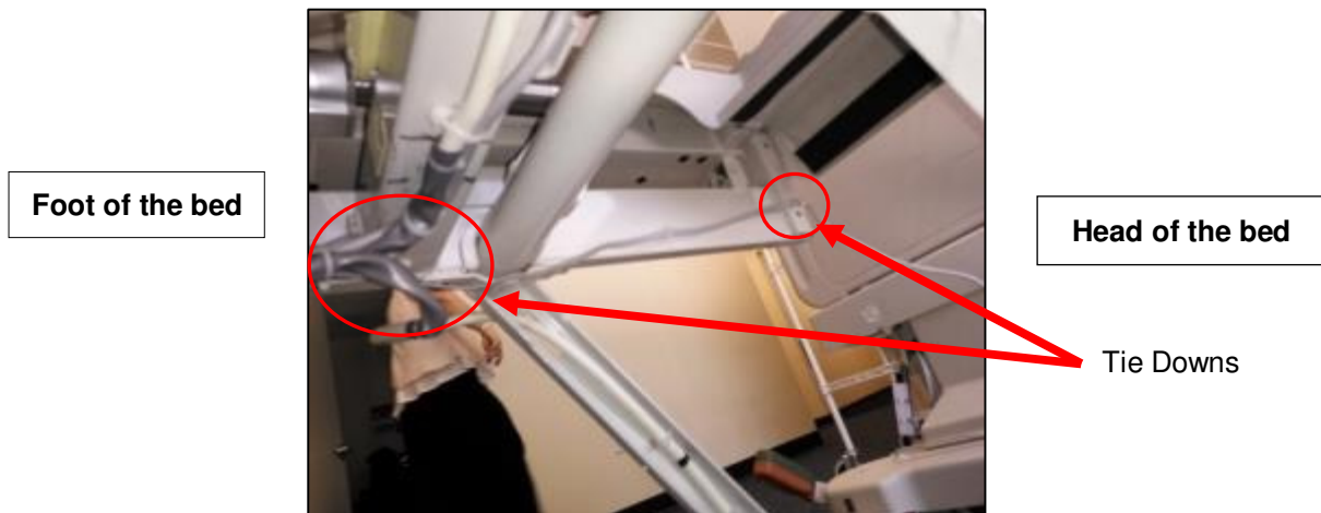
Figure 9. AC Line Power Sensor Cable Routing and Cable Tie Holder Placement
