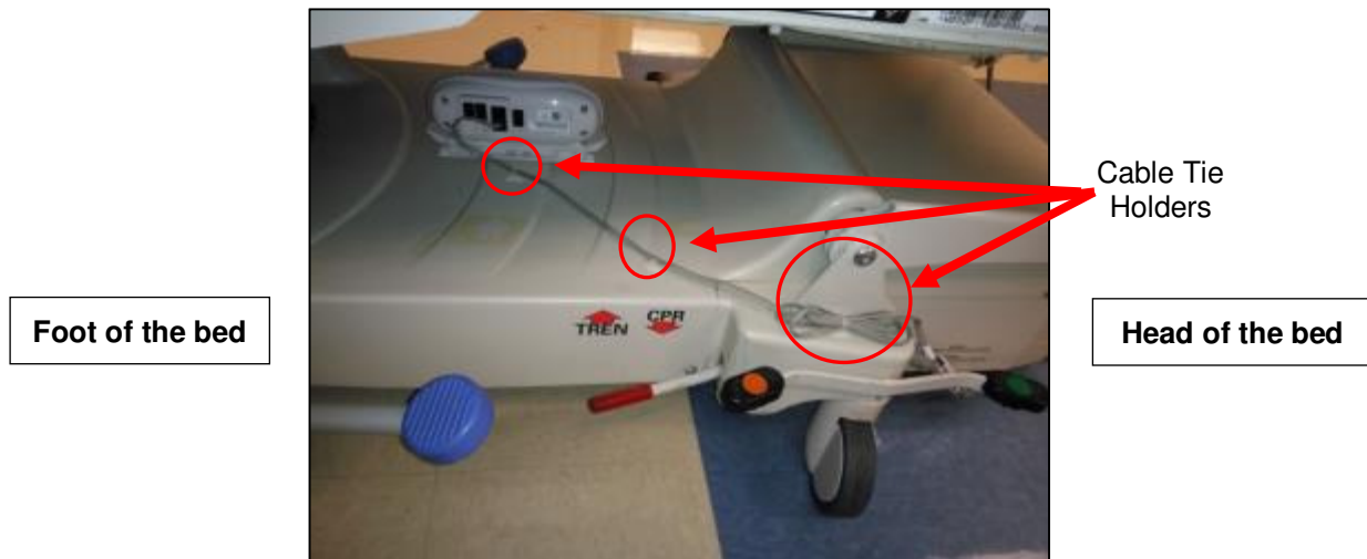
Figure 6. AC Line Power Sensor Cable Routing
