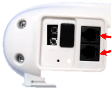
Figure 3. Connecting the AC Line Power Sensor to the Bed Beacon via the RJ11 connector
