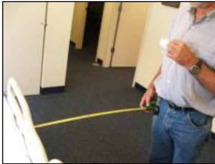
Figure 13. Test Badge Activation Distance from Bed's Handrail Center is 18" (at edge for stretcher installations)
