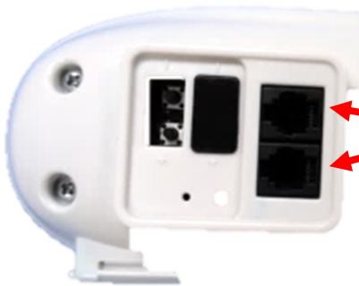
Figure 4. Connecting the AC Line Power Sensor to the Bed Beacon via the RJ11 connector
