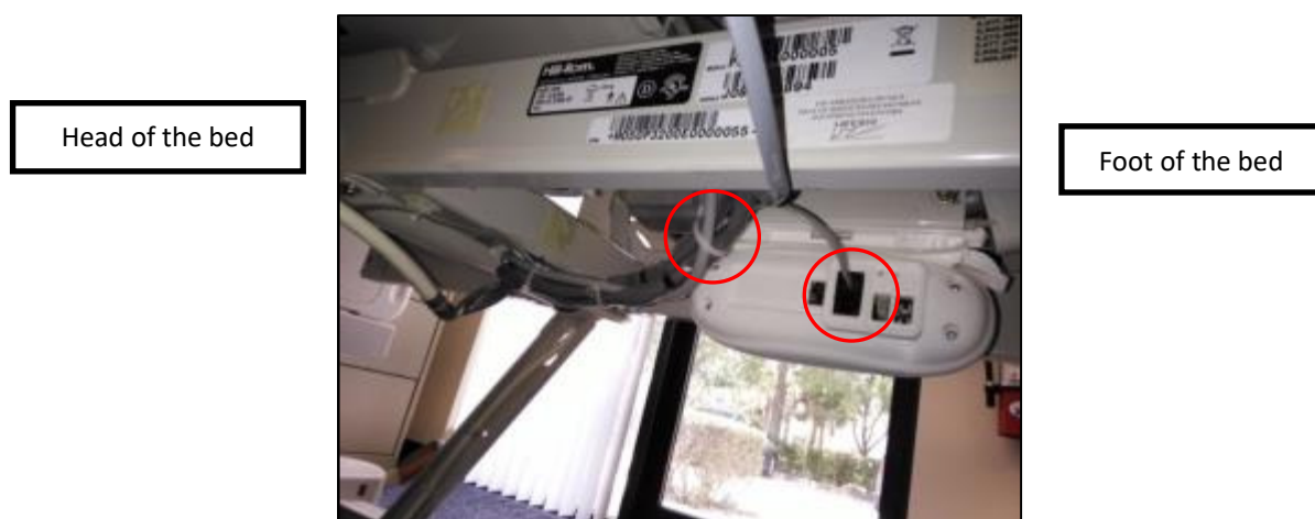
Figure 10. AC Line Power Sensor Cable Routing to Bed Beacon and Cable Tie Holder Placement
