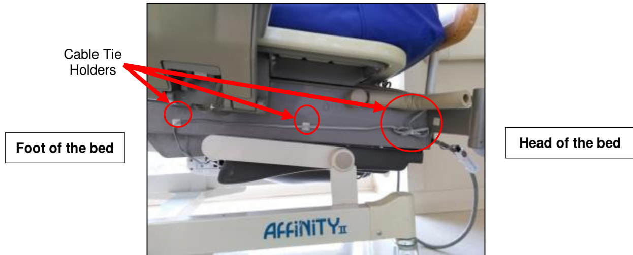
Figure 5. AC Line Power Sensor Cable Routing
