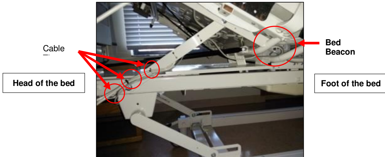
Figure 5. AC Line Power Sensor Cable Routing
