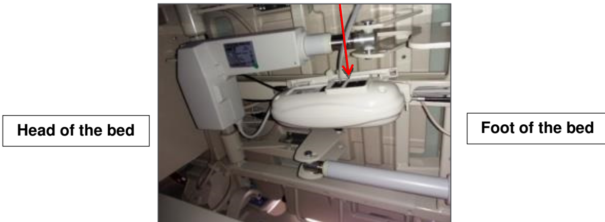
Figure 1. Bed Beacon Installation Location
