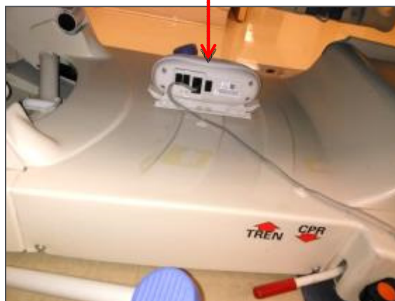
Figure 1 & 2. Bed Beacon Installation Location on the Bed
