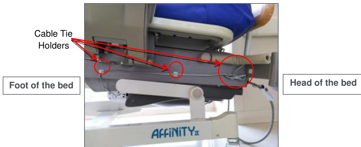
Figure 5. AC Line Power Sensor Cable Routing
