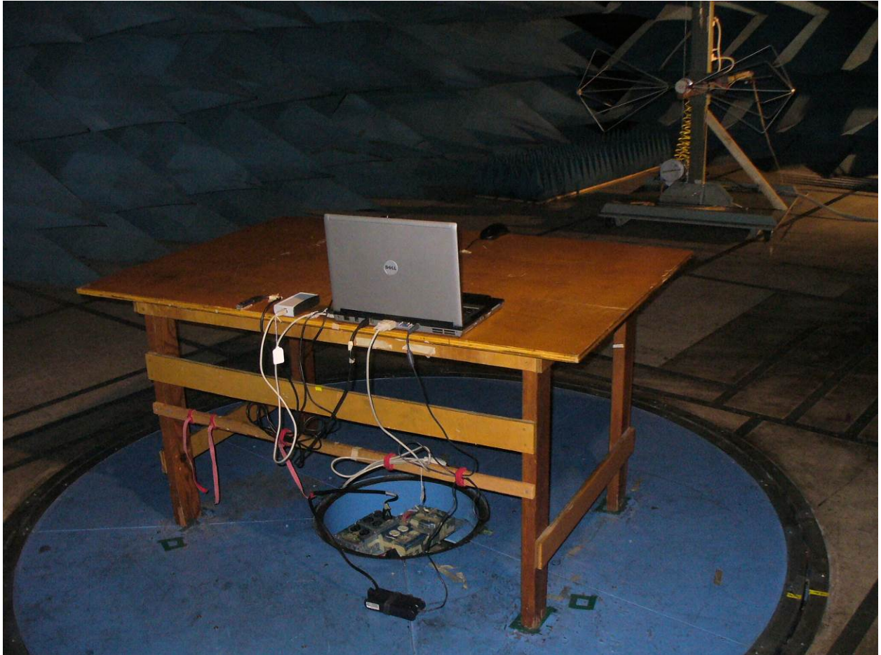
Figure 3: Radiated Emissions – Back View 2 – 30 MHz – 200 MHz
