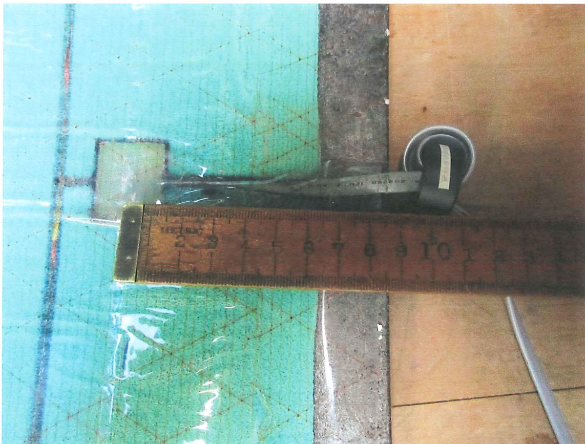
Figure A1: FAIR-RITE Part# 2643866402 Ferrite on Antenna Cable (4 Passes) – View 1
