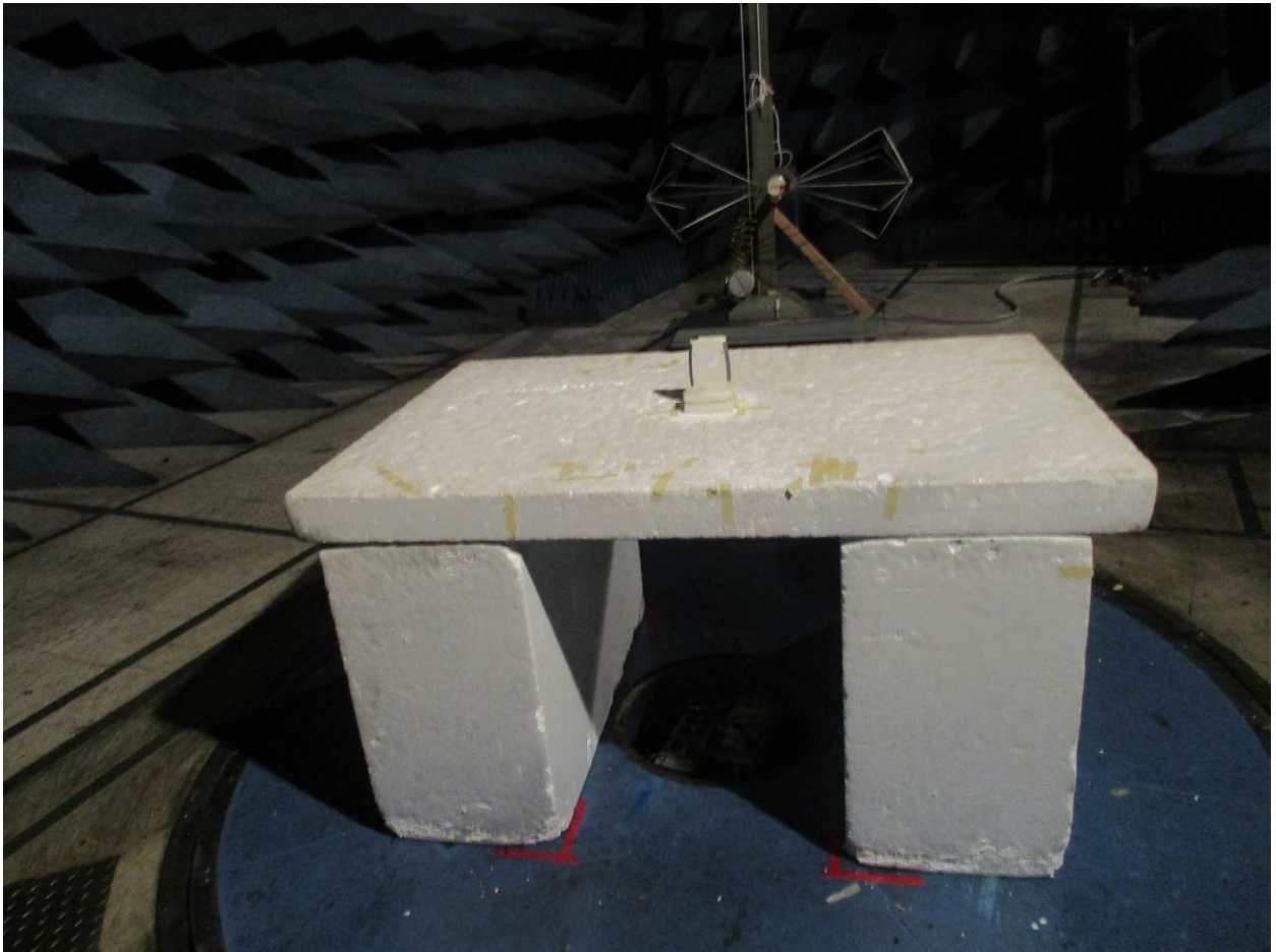
Figure 3: Radiated Emissions – Back View – 30 MHz – 200 MHz (EUT Standing)
