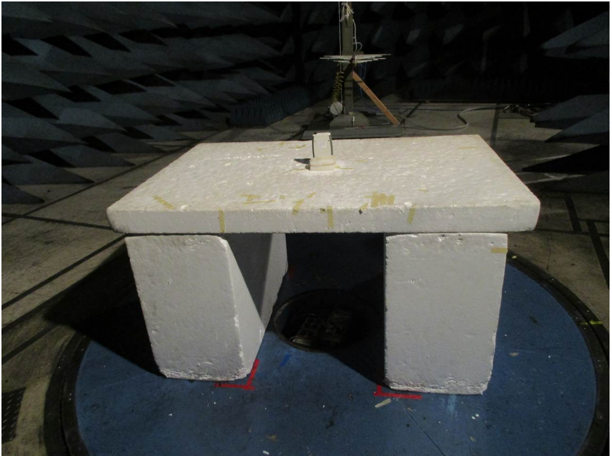
Figure 4: Radiated Emissions – Back View – 200 MHz – 1 GHz (EUT Standing)
