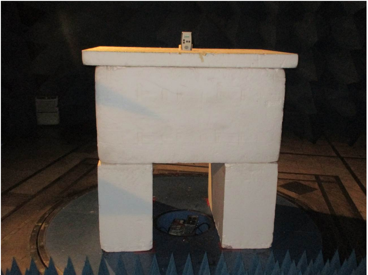
Figure 5: Radiated Emissions – Front View – Above 1 GHz (EUT Standing)
