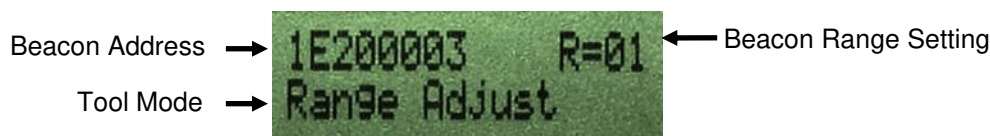
Figure 11 – Display in Range Adjust Mode, System B
