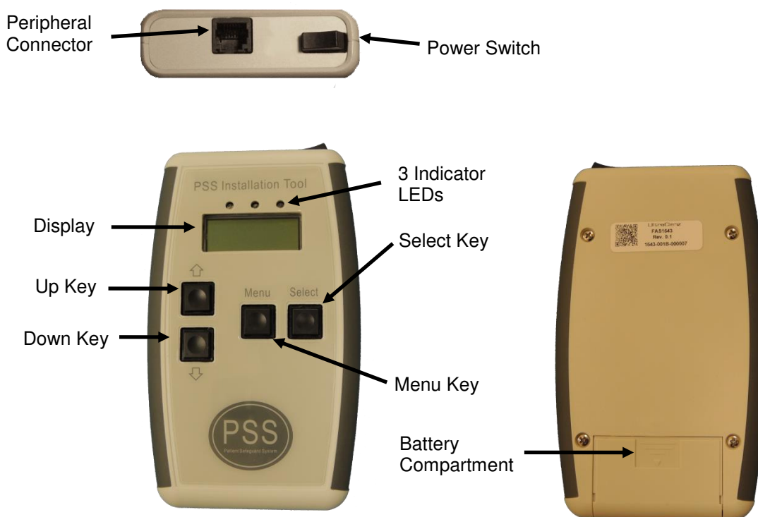
Figure 1 - FAS1543 Beacon Installation Tool's Features
