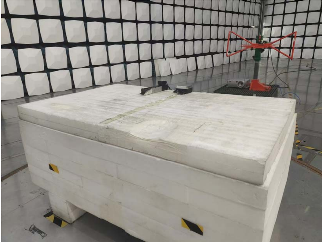
Radiated Emissions Below 1G side View
