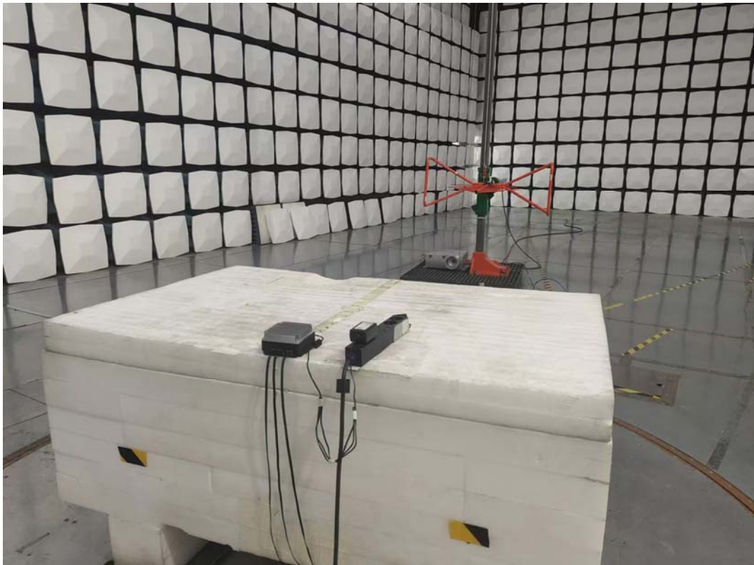
Radiated Emissions Below 1G side View
