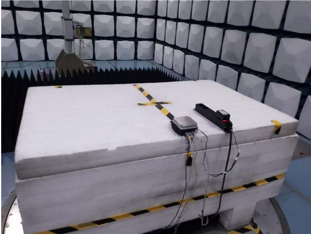
Radiated Emissions 1-18G View
