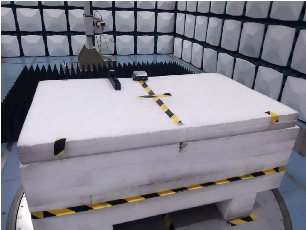
Radiated Emissions 18-26.5G View
