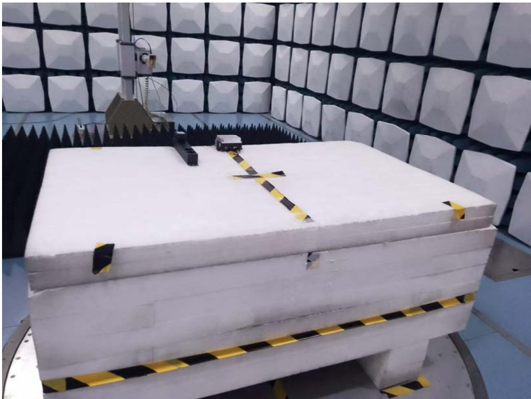
Radiated Emissions 26.5-30G View
