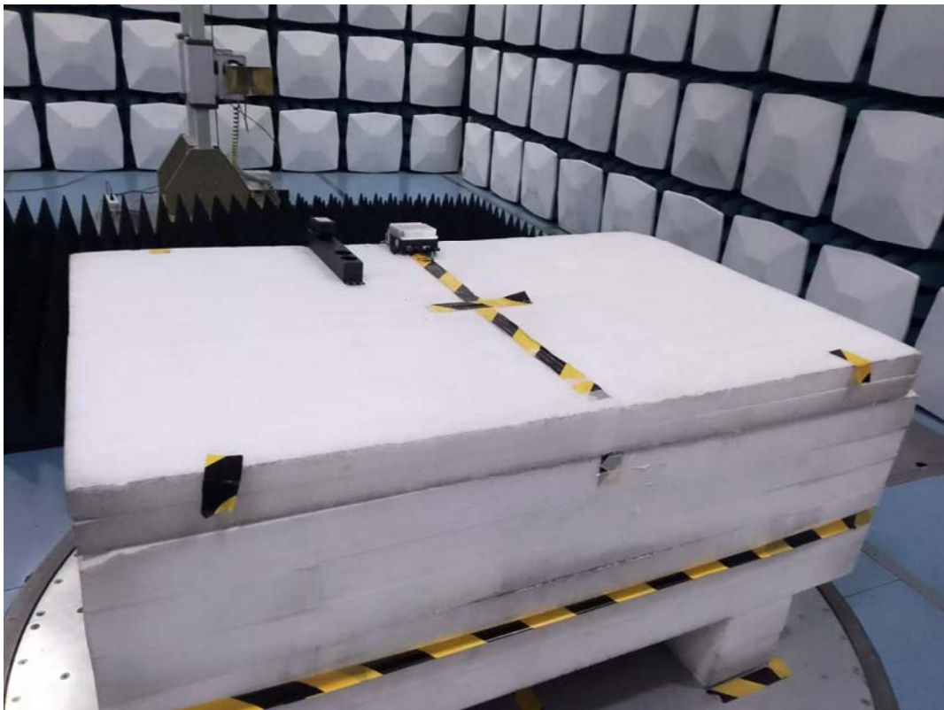
Radiated Emissions 1-18G View
