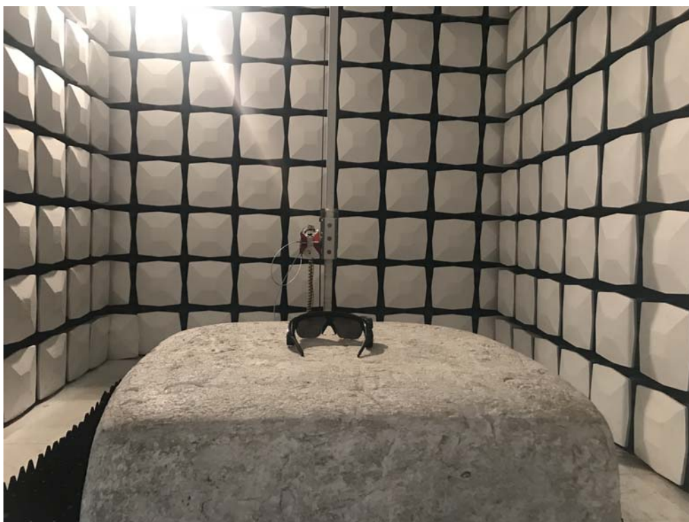
Description: Radiated Emission Test Setup for 1~18GHz
