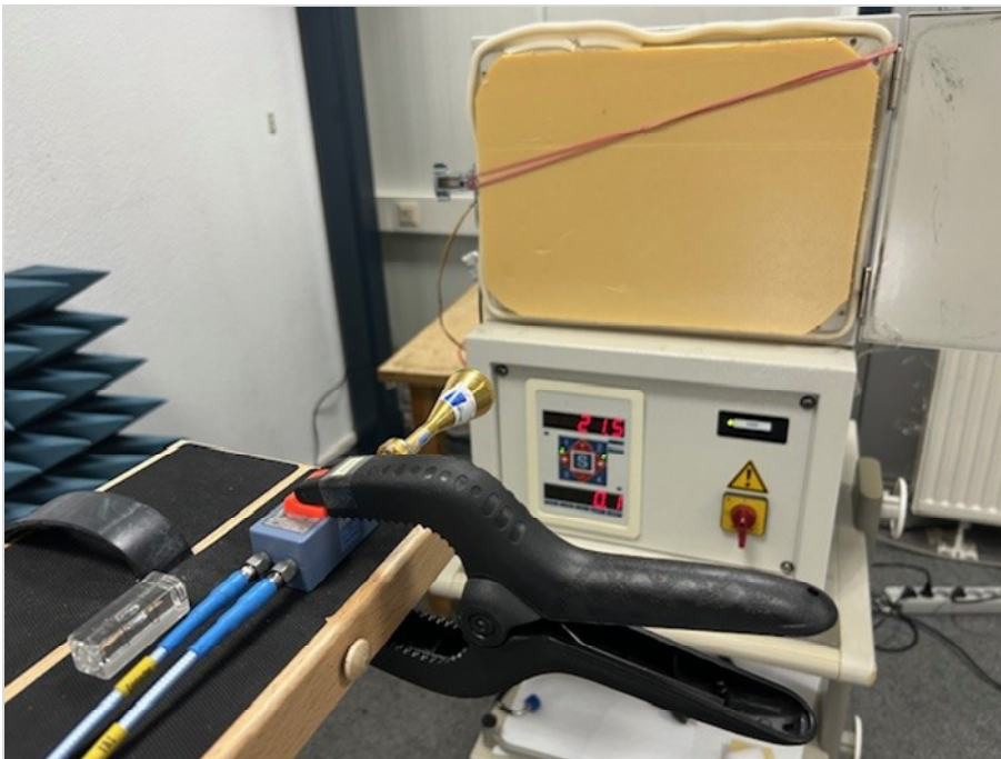
Photograph 10: EUT test setup in the RC8G Lab_climate cabinet
