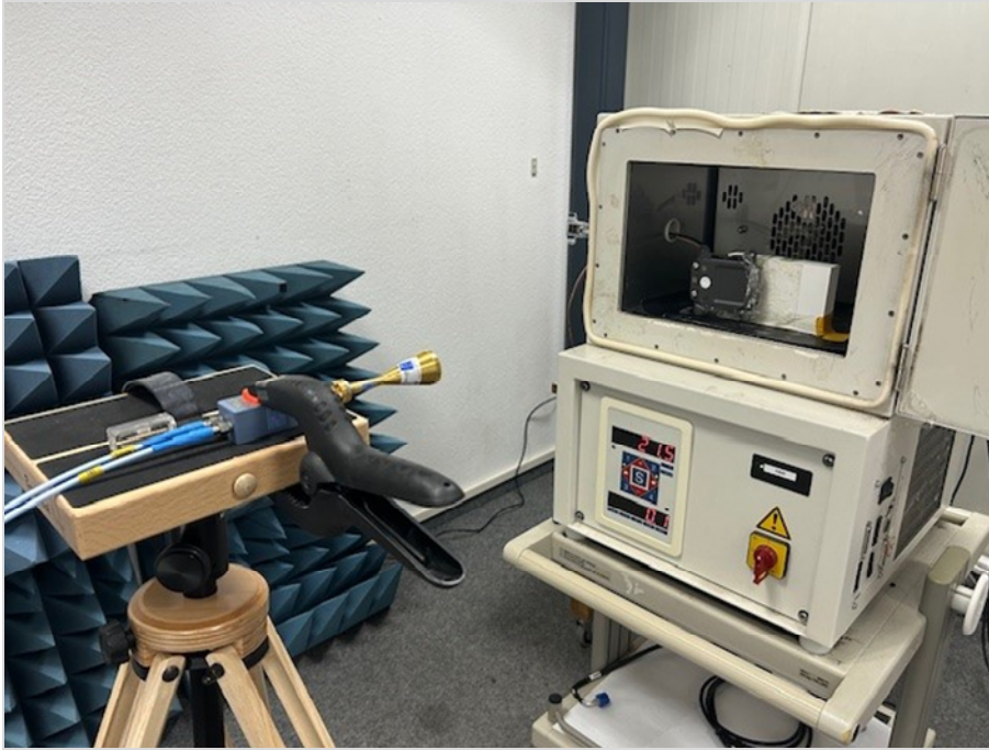
Photograph 9: EUT test setup in the RC8G Lab_climate cabinet
