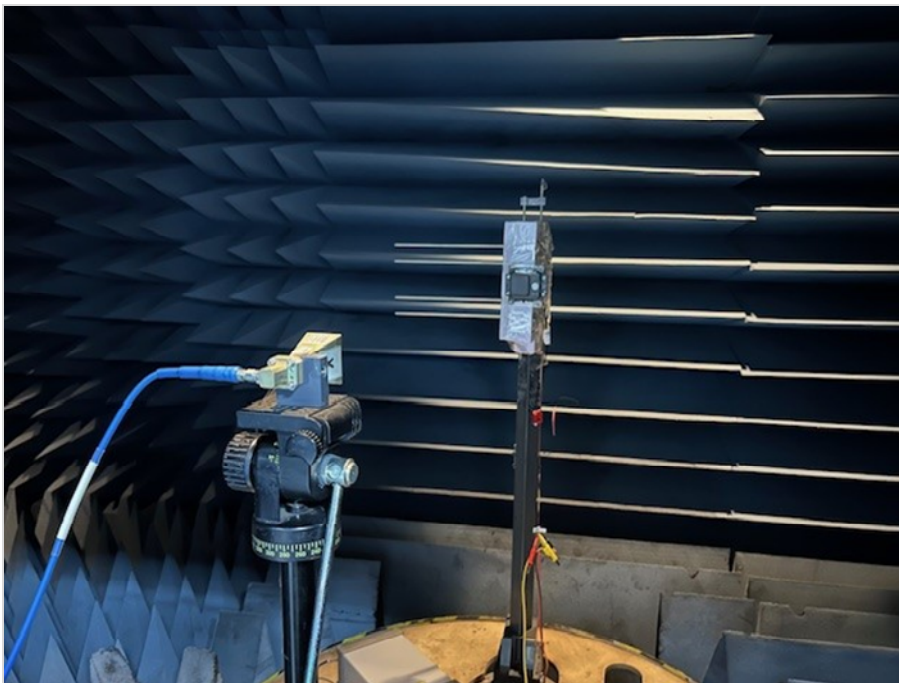
Photograph 8: EUT test setup in the fully anechoic chamber (FAC2)
