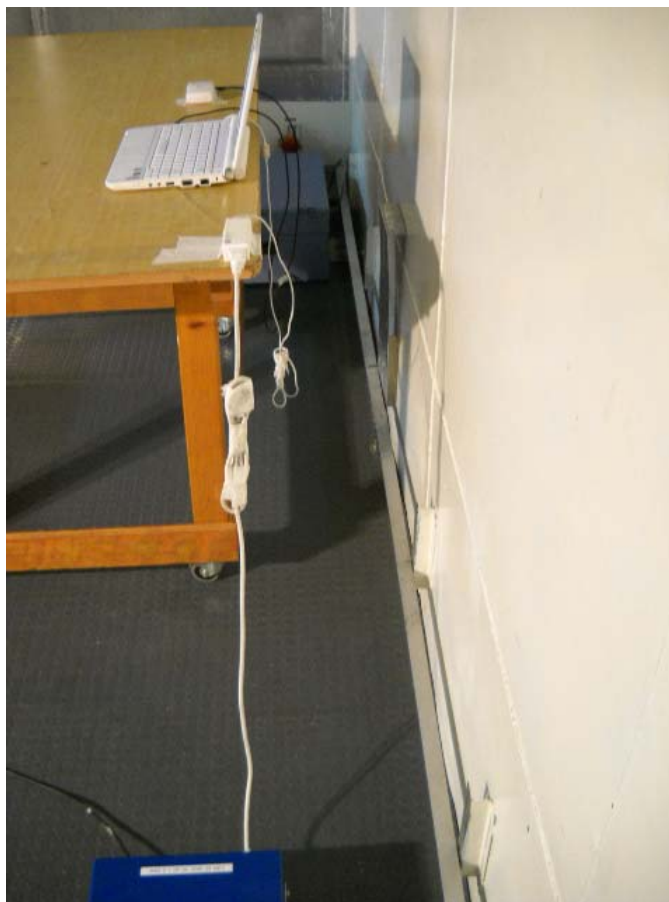
Photograph 8.1.2 Setup for conducted emission measurements
