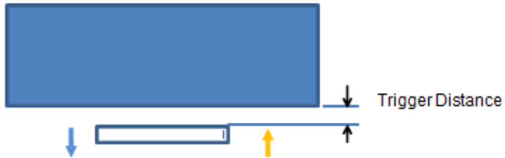
Picture: Proximity sensor triggering distances assessment (Back)
