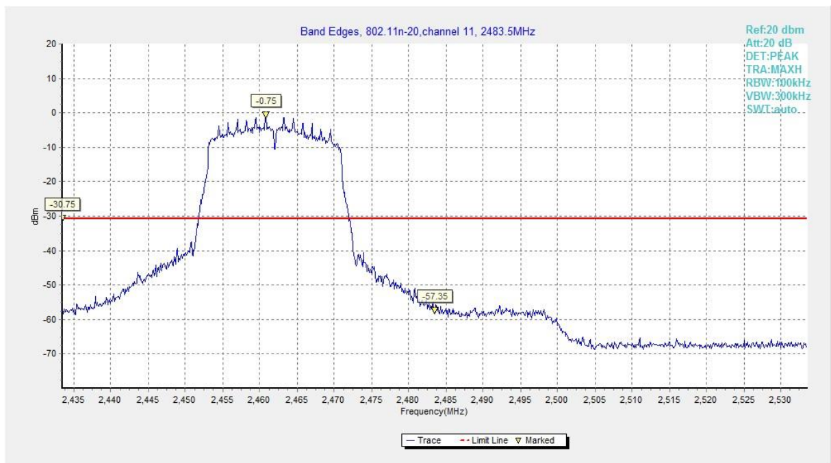
Fig.30 Band Edges (802.11n HT20, CH 11)
