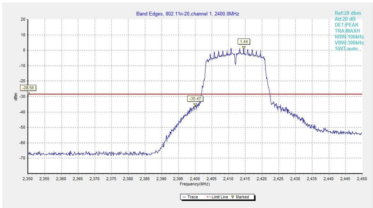
Fig.29 Band Edges (802.11n HT20, CH 1)
