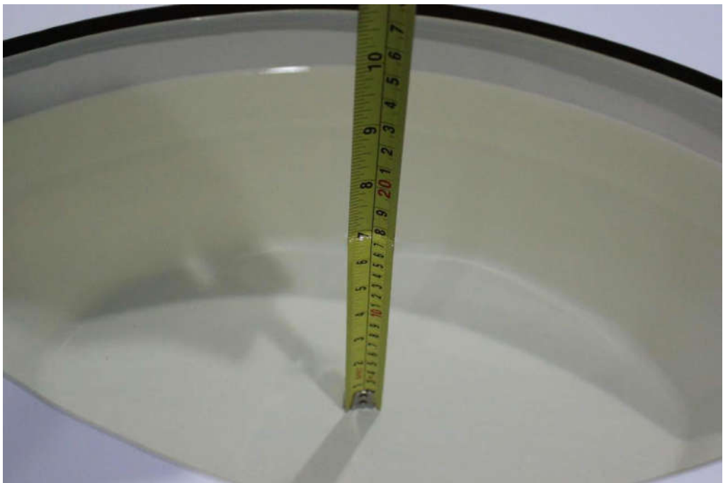
Picture 7-6: Liquid depth in the Flat Phantom(5GHz)
